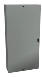
Hammond Eclipse series enclosure, NEMA 3R/4/12, 72 x 36 x 12in (HxWxD), wall mount, carbon steel, ANSI 61 gray, powder coat finish, single-door, 3-point keylocking handle.
