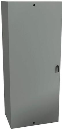
Hammond Eclipse series enclosure, NEMA 3R/4/12, 72 x 30 x 20in (HxWxD), wall mount, carbon steel, ANSI 61 gray, powder coat finish, single-door, 3-point keylocking handle.
