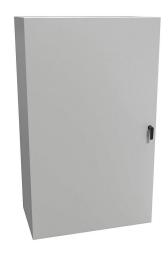
Hammond Eclipse series enclosure, NEMA 3R/4/12, 60 x 36 x 20in (HxWxD), wall mount, carbon steel, RAL 7035 light gray, powder coat finish, single-door, 3-point keylocking handle.
