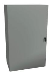
Hammond Eclipse series enclosure, NEMA 3R/4/12, 60 x 36 x 20in (HxWxD), wall mount, carbon steel, ANSI 61 gray, powder coat finish, single-door, 3-point keylocking handle.
