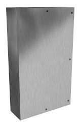
Hammond Eclipse series enclosure, NEMA 3R/4/4X/12/13,  $60 \times 36 \times 12$  in (HxWxD), wall mount, 316 stainless steel, #4 brush finish, single-door, 1/4-turn semi-flush 316 stainless steel latch.
