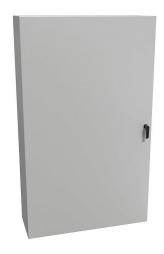
Hammond Eclipse series enclosure, NEMA 3R/4/12, 60 x 36 x 12in (HxWxD), wall mount, carbon steel, RAL 7035 light gray, powder coat finish, single-door, 3-point keylocking handle.
