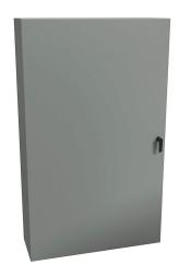
Hammond Eclipse series enclosure, NEMA 3R/4/12, 60 x 36 x 12in (HxWxD), wall mount, carbon steel, ANSI 61 gray, powder coat finish, single-door, 3-point keylocking handle.
