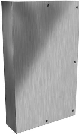
Hammond Eclipse series enclosure, NEMA 3R/4/4X/12/13, 60 x 36 x 10in (HxWxD), wall mount, 304 stainless steel, #4 brush finish, single-door, 1/4-turn semi-flush 316 stainless steel latch.
