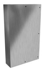
Hammond Eclipse series enclosure, NEMA 3R/4/4X/12/13,  $60 \times 36 \times 10$  in (HxWxD), wall mount, 304 stainless steel, #4 brush finish, single-door, 1/4-turn semi-flush 316 stainless steel latch.
