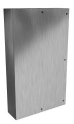
Hammond Eclipse series enclosure, NEMA 3R/4/4X/12/13, 60 x 36 x 10in (HxWxD), wall mount, 316 stainless steel, #4 brush finish, single-door, 1/4-turn semi-flush 316 stainless steel latch.
