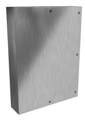
Hammond Eclipse series enclosure, NEMA 3R/4/4X/12/13, 48 x 36 x 8in (HxWxD), wall mount, 304 stainless steel, #4 brush finish, single-door, 1/4-turn semi-flush 316 stainless steel latch.
