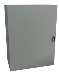
Hammond Eclipse series enclosure, NEMA 3R/4/12, 48 x 36 x 20in (HxWxD), wall mount, carbon steel, ANSI 61 gray, powder coat finish, single-door, 3-point keylocking handle.
