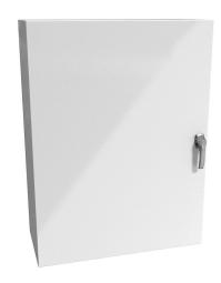
Hammond Eclipse series enclosure, NEMA 3R/4/4X/12/13,  $48 \times 36 \times 16$  in (HxWxD), wall mount, 304 stainless steel, RAL 9003 white, powder coat finish, single-door, 3-point 316 stainless steel padlocking handle.
