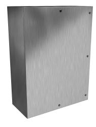
Hammond Eclipse series enclosure, NEMA 3R/4/4X/12/13, 48 x 36 x 16in (HxWxD), wall mount, 316 stainless steel, #4 brush finish, single-door, 1/4-turn semi-flush 316 stainless steel latch.
