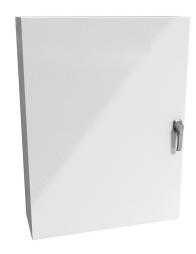
Hammond Eclipse series enclosure, NEMA 3R/4/4X/12/13,  $48 \times 36 \times 12$  in (HxWxD), wall mount, 304 stainless steel, RAL 9003 white, powder coat finish, single-door, 3-point 316 stainless steel padlocking handle.
