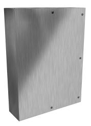
Hammond Eclipse series enclosure, NEMA 3R/4/4X/12/13, 48 x 36 x 10in (HxWxD), wall mount, 304 stainless steel, #4 brush finish, single-door, 1/4-turn semi-flush 316 stainless steel latch.
