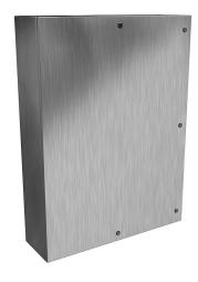
Hammond Eclipse series enclosure, NEMA 3R/4/4X/12/13,  $48 \times 36 \times 10$  in (HxWxD), wall mount, 316 stainless steel, #4 brush finish, single-door, 1/4-turn semi-flush 316 stainless steel latch.
