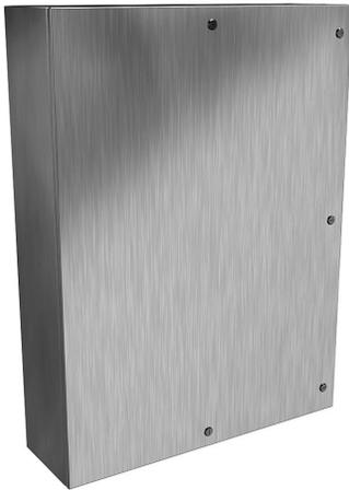
Hammond Eclipse series enclosure, NEMA 3R/4/4X/12/13, 48 x 36 x 10in (HxWxD), wall mount, 316 stainless steel, #4 brush finish, single-door, 1/4-turn semi-flush 316 stainless steel latch.
