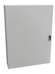
Hammond Eclipse series enclosure, NEMA 3R/4/12, 48 x 36 x 10in (HxWxD), wall mount, carbon steel, RAL 7035 light gray, powder coat finish, single-door, 3-point keylocking handle.
