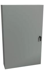
Hammond Eclipse series enclosure, NEMA 3R/4/12, 48 x 30 x 8in (HxWxD), wall mount, carbon steel, ANSI 61 gray, powder coat finish, single-door, 3-point keylocking handle.
