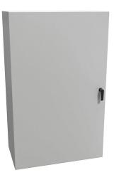
Hammond Eclipse series enclosure, NEMA 3R/4/12, 48 x 30 x 16in (HxWxD), wall mount, carbon steel, RAL 7035 light gray, powder coat finish, single-door, 3-point keylocking handle.
