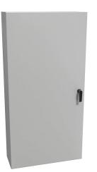
Hammond Eclipse series enclosure, NEMA 3R/4/12, 48 x 24 x 8in (HxWxD), wall mount, carbon steel, RAL 7035 light gray, powder coat finish, single-door, 3-point keylocking handle.
