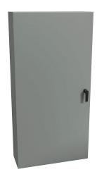
Hammond Eclipse series enclosure, NEMA 3R/4/12, 48 x 24 x 8in (HxWxD), wall mount, carbon steel, ANSI 61 gray, powder coat finish, single-door, 3-point keylocking handle.
