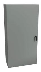
Hammond Eclipse series enclosure, NEMA 3R/4/12, 48 x 24 x 12in (HxWxD), wall mount, carbon steel, ANSI 61 gray, powder coat finish, single-door, 3-point keylocking handle.
