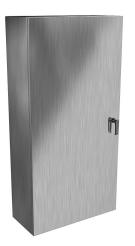
Hammond Eclipse series enclosure, NEMA 3R/4/4X/12/13, 48 x 24 x 10in (HxWxD), wall mount, 304 stainless steel, #4 brush finish, single-door, 3-point keylocking handle.
