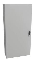
Hammond Eclipse series enclosure, NEMA 3R/4/12, 48 x 24 x 10in (HxWxD), wall mount, carbon steel, RAL 7035 light gray, powder coat finish, single-door, 3-point keylocking handle.
