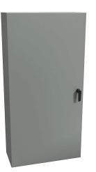
Hammond Eclipse series enclosure, NEMA 3R/4/12, 48 x 24 x 10in (HxWxD), wall mount, carbon steel, ANSI 61 gray, powder coat finish, single-door, 3-point keylocking handle.
