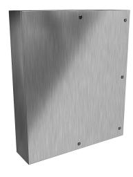
Hammond Eclipse series enclosure, NEMA 3R/4/4X/12/13,  $42 \times 36 \times 8$  in (HxWxD), wall mount, 304 stainless steel, #4 brush finish, single-door, 1/4-turn semi-flush 316 stainless steel latch.
