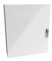
Hammond Eclipse series enclosure, NEMA 3R/4/4X/12/13,  $42 \times 36 \times 12$  in (HxWxD), wall mount, 304 stainless steel, RAL 9003 white, powder coat finish, single-door, 3-point 316 stainless steel padlocking handle.
