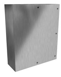
Hammond Eclipse series enclosure, NEMA 3R/4/4X/12/13,  $42 \times 36 \times 12$  in (HxWxD), wall mount, 304 stainless steel, #4 brush finish, single-door, 1/4-turn semi-flush 316 stainless steel latch.
