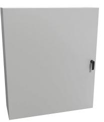
Hammond Eclipse series enclosure, NEMA 3R/4/12, 42 x 36 x 12in (HxWxD), wall mount, carbon steel, RAL 7035 light gray, powder coat finish, single-door, 3-point keylocking handle.
