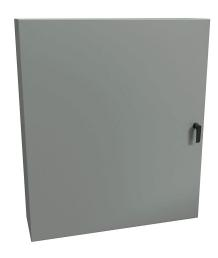
Hammond Eclipse series enclosure, NEMA 3R/4/12, 42 x 36 x 10in (HxWxD), wall mount, carbon steel, ANSI 61 gray, powder coat finish, single-door, 3-point keylocking handle.
