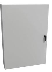
Hammond Eclipse series enclosure, NEMA 3R/4/12, 42 x 30 x 8in (HxWxD), wall mount, carbon steel, RAL 7035 light gray, powder coat finish, single-door, 3-point keylocking handle.
