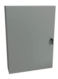
Hammond Eclipse series enclosure, NEMA 3R/4/12,  $42 \times 30 \times 8in$  (HxWxD), wall mount, carbon steel, ANSI 61 gray, powder coat finish, single-door, 3-point keylocking handle.
