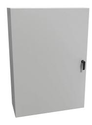
Hammond Eclipse series enclosure, NEMA 3R/4/12, 42 x 30 x 12in (HxWxD), wall mount, carbon steel, RAL 7035 light gray, powder coat finish, single-door, 3-point keylocking handle.
