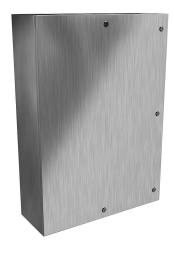
Hammond Eclipse series enclosure, NEMA 3R/4/4X/12/13,  $42 \times 30 \times 10$  in (HxWxD), wall mount, 304 stainless steel, #4 brush finish, single-door, 1/4-turn semi-flush 316 stainless steel latch.
