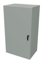
Hammond Eclipse series enclosure, NEMA 3R/4/12, 42 x 24 x 16in (HxWxD), wall mount, carbon steel, ANSI 61 gray, powder coat finish, single-door, 3-point keylocking handle.
