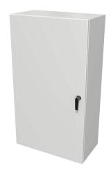
Hammond Eclipse series enclosure, NEMA 3R/4/12, 42 x 24 x 12in (HxWxD), wall mount, carbon steel, RAL 7035 light gray, powder coat finish, single-door, 3-point keylocking handle.
