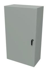
Hammond Eclipse series enclosure, NEMA 3R/4/12, 42 x 24 x 12in (HxWxD), wall mount, carbon steel, ANSI 61 gray, powder coat finish, single-door, 3-point keylocking handle.
