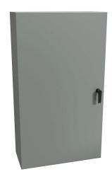
Hammond Eclipse series enclosure, NEMA 3R/4/12, 42 x 24 x 10in (HxWxD), wall mount, carbon steel, ANSI 61 gray, powder coat finish, single-door, 3-point keylocking handle.
