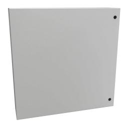
Hammond Eclipse series enclosure, NEMA 3R/4/12, 36 x 36 x 8in (HxWxD), wall mount, carbon steel, RAL 7035 light gray, powder coat finish, single-door, 1/4-turn semi-flush latch.
