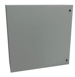
Hammond Eclipse series enclosure, NEMA 3R/4/12, 36 x 36 x 12in (HxWxD), wall mount, carbon steel, ANSI 61 gray, powder coat finish, single-door, 1/4-turn semi-flush latch.
