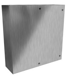
Hammond Eclipse series enclosure, NEMA 3R/4/4X/12/13,  $36 \times 36 \times 10$  in (HxWxD), wall mount, 304 stainless steel, #4 brush finish, single-door, 1/4-turn semi-flush 316 stainless steel latch.
