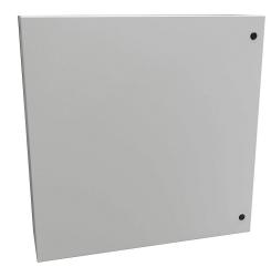
Hammond Eclipse series enclosure, NEMA 3R/4/12,  $36 \times 36 \times 10$ in (HxWxD), wall mount, carbon steel, RAL 7035 light gray, powder coat finish, single-door, 1/4-turn semi-flush latch.
