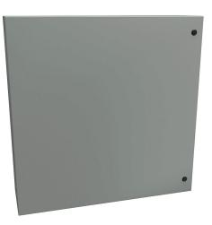
Hammond Eclipse series enclosure, NEMA 3R/4/12, 36 x 36 x 10in (HxWxD), wall mount, carbon steel, ANSI 61 gray, powder coat finish, single-door, 1/4-turn semi-flush latch.
