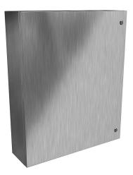
Hammond Eclipse series enclosure, NEMA 3R/4/4X/12/13, 36 x 30 x 8in (HxWxD), wall mount, 304 stainless steel, #4 brush finish, single-door, 1/4-turn semi-flush 316 stainless steel latch.
