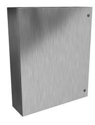
Hammond Eclipse series enclosure, NEMA 3R/4/4X/12/13, 36 x 30 x 8in (HxWxD), wall mount, 316 stainless steel, #4 brush finish, single-door, 1/4-turn semi-flush 316 stainless steel latch.
