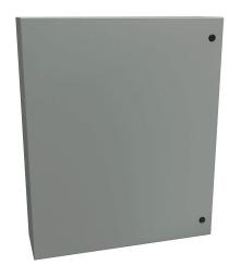
Hammond Eclipse series enclosure, NEMA 3R/4/12,  $36 \times 30 \times 8in$  (HxWxD), wall mount, carbon steel, ANSI 61 gray, powder coat finish, single-door, 1/4-turn semi-flush latch.
