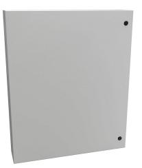
Hammond Eclipse series enclosure, NEMA 3R/4/12,  $36 \times 30 \times 6in$  (HxWxD), wall mount, carbon steel, RAL 7035 light gray, powder coat finish, single-door, 1/4-turn semi-flush latch.
