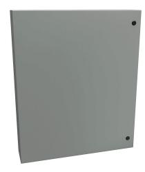
Hammond Eclipse series enclosure, NEMA 3R/4/12,  $36 \times 30 \times 6$ in (HxWxD), wall mount, carbon steel, ANSI 61 gray, powder coat finish, single-door, 1/4-turn semi-flush latch.
