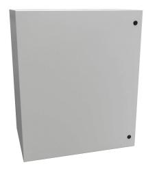
Hammond Eclipse series enclosure, NEMA 3R/4/12,  $36 \times 30 \times 20$ in (HxWxD), wall mount, carbon steel, RAL 7035 light gray, powder coat finish, single-door, 1/4-turn semi-flush latch.
