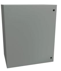
Hammond Eclipse series enclosure, NEMA 3R/4/12, 36 x 30 x 20in (HxWxD), wall mount, carbon steel, ANSI 61 gray, powder coat finish, single-door, 1/4-turn semi-flush latch.
